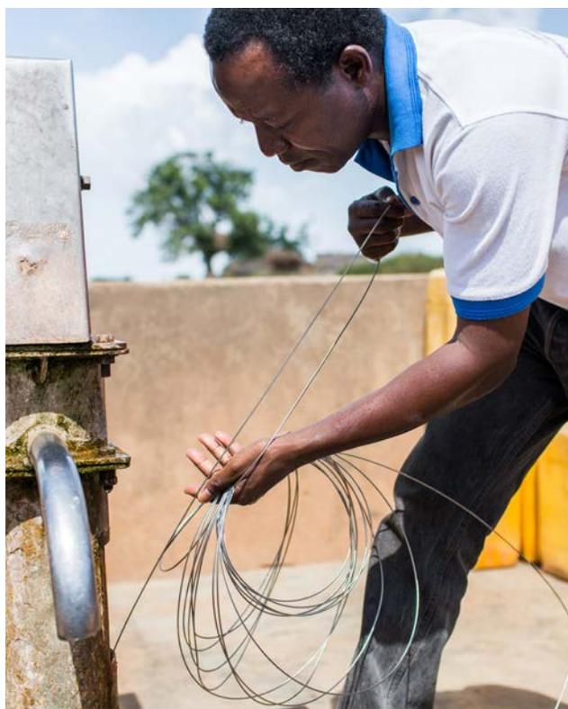
**WaterAid Burkina Faso's Regional Learning Center Coordinator, Lucien Damiba, removes a water monitoring device from a borehole.**
